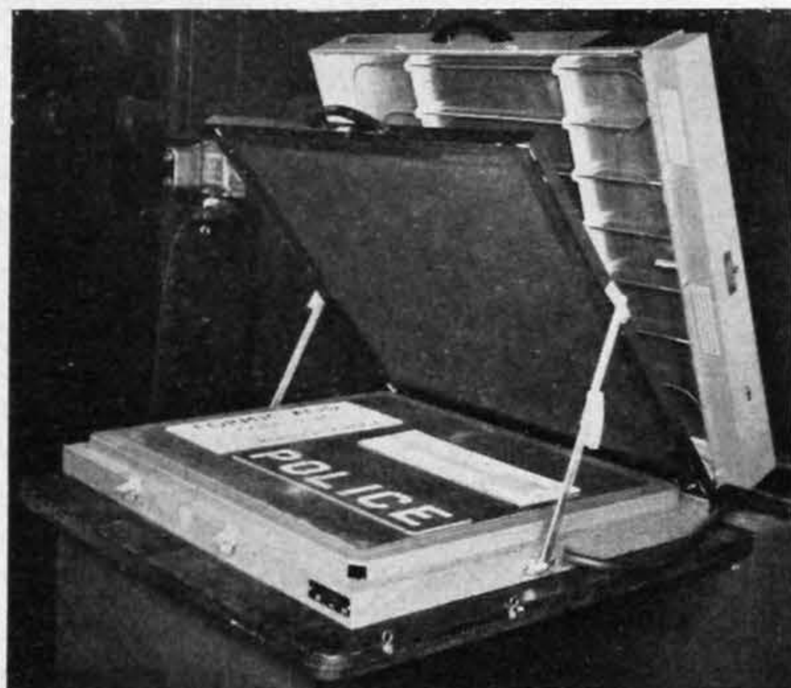
A small plant for the rapid manufacture of permanent, day-and-night signs
