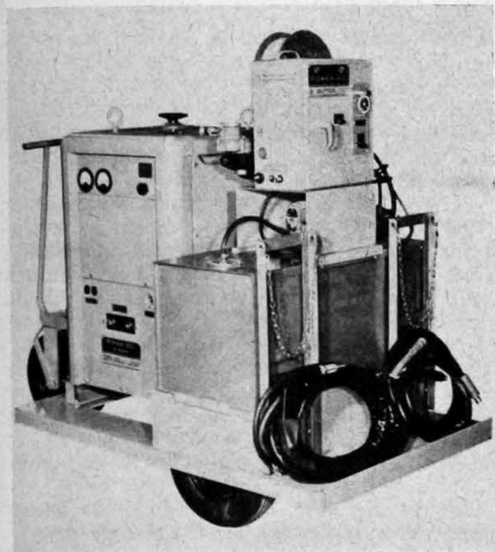
Mobile equipment for automatic and semi-automatic gas-shielded, consumable electrode welding
