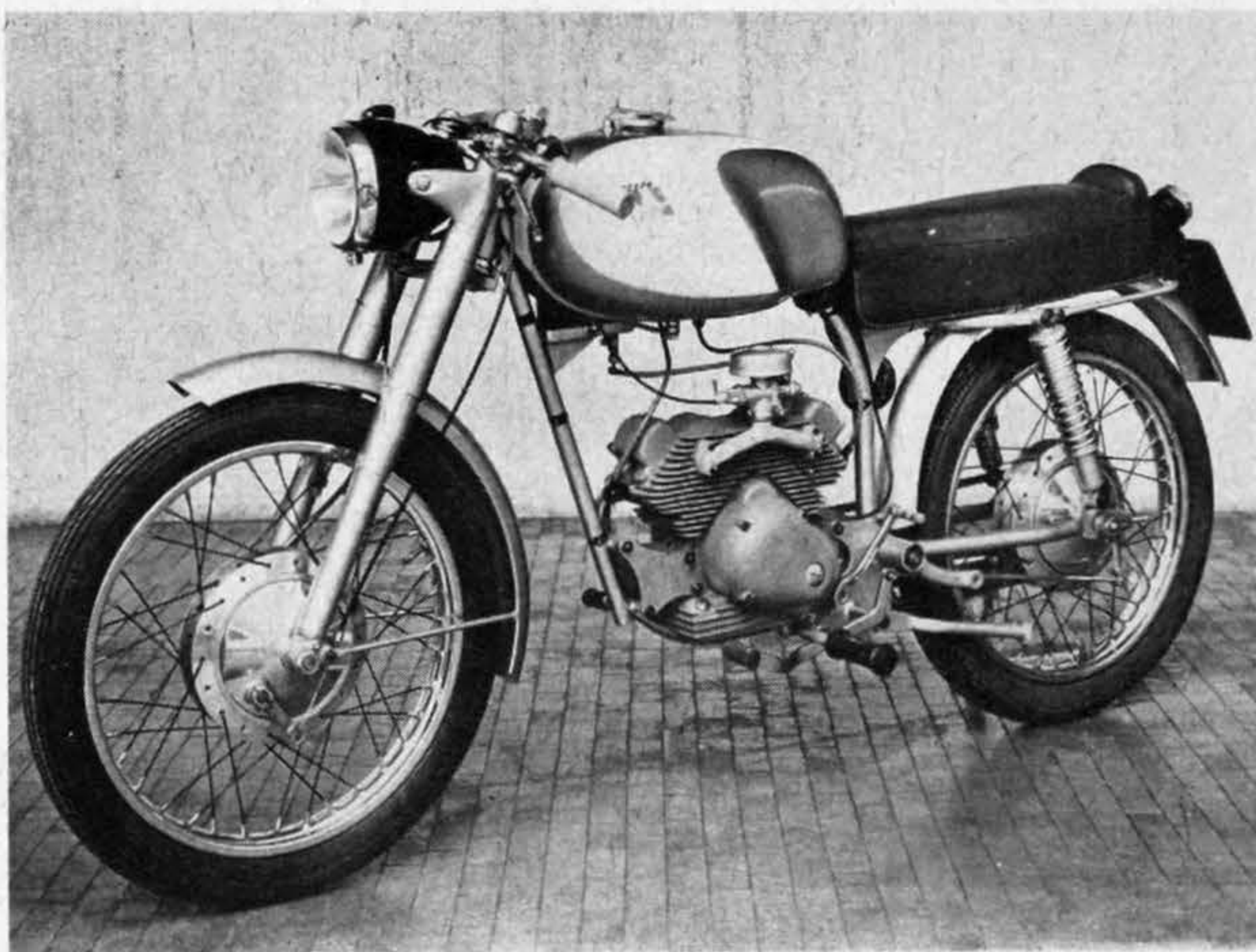
The 90 deg. V-twin engine of the "La Strada" has a single carburetter. In the lightness of the cycle parts the machine is typical of Italian design
