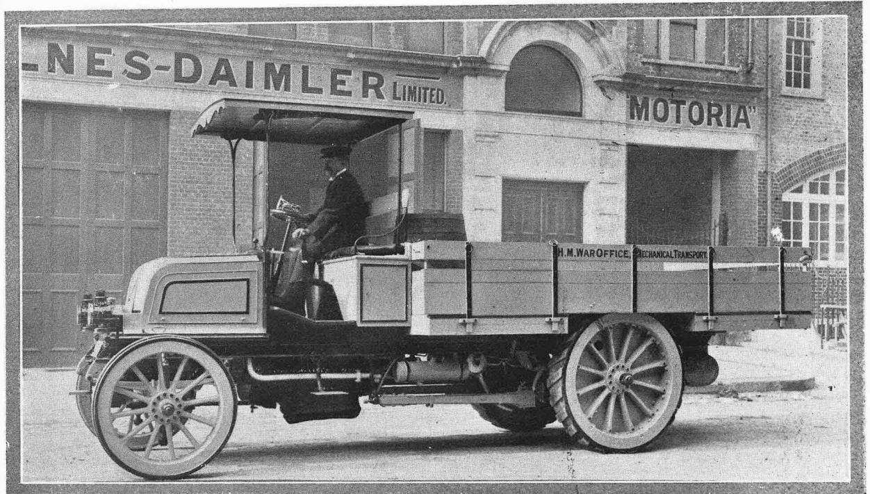
A WAR OFFICE LORRY. The lorry illustrated above is one of two which the Milnes-Daimler have supplied to the War Office for transport service. Petrol engines supply the tractive power, the transmission being on the company's now well-known system.
