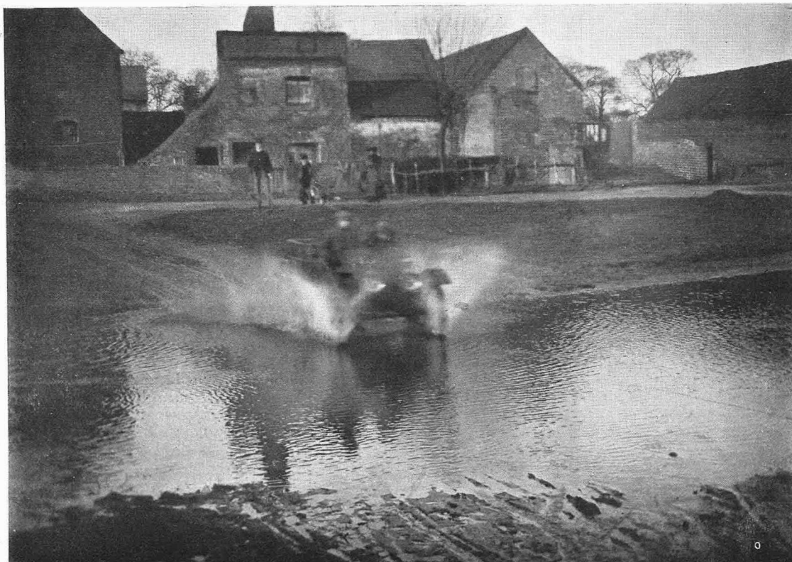
This illustration was taken during a series of experiments with a Lanchester car, to prove that it was not affected by wet, whether from above or thrown up from the road. The machine was driven repeatedly through a ford of a river in the Midlands, at speeds varying from twenty to thirty miles an hour. Water was thrown up the sloping dash of the car in a solid wave, and the occupants were soaked to the skin. The test showed that the motor ran just as well though absolutely waterlogged, and proved conclusively that the mechanism was waterproof in the true sense of the word.
