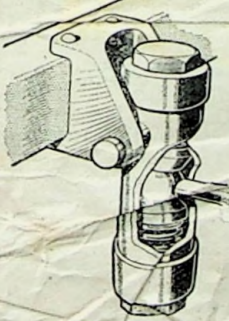
The illustration below shows in detail the forward anchorage of the torque stay depicted on the right. The rod is ball-ended and the bearing is spring-loaded.
