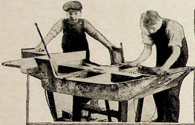
There are two distinct stages in the building of the Austin Seven body. The first is the construction of a sheet-metal framework, shown above, and the second the attachment of the aluminium panel to it, with the result shown in the top right picture. The bottom photograph shows the body being flow-painted.
