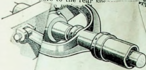
An alternative method to that shown in the adjacent illustration, anchoring the forward end of a torque tube. So the fork is anchored direct to the gearbox.
