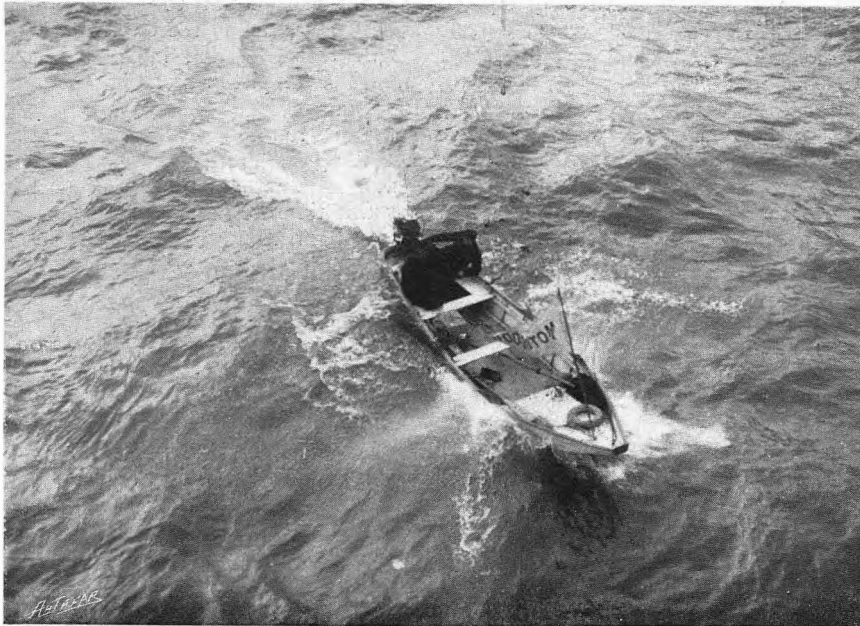
The Motogodille in choppy water. This is an ordinary type of craft with the motor mounted over the rudder.
