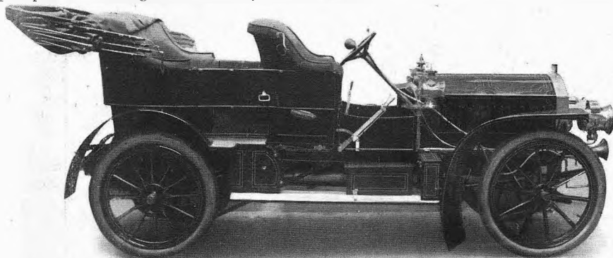
A six-cylinder 40 h.p. Napier, built for Mr. F. J. Cullinan. This car is intended for use in South Africa, and several deviations have, therefore, been made from the English standard. The wheels are 40in. in diameter, and the springs are placed well above the axles, which are of special shape, thus giving no less than 2in. from the engine cover to the ground. On account of the frequent necessity to cross deep spruets, etc., the exhaust outlet is placed very high up. The body is built chiefly of aluminium, and carries five passengers.
