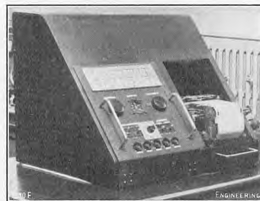
FIG. 6. AUTOMATIC RECORDER FOR STRAIN GAUGES.
