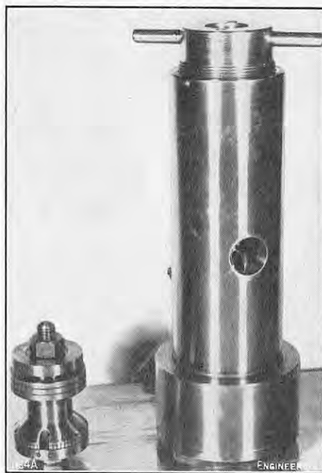
FIG. 1. MACHINE FOR VIBRATION TESTING OF NUTS AND BOLTS.
