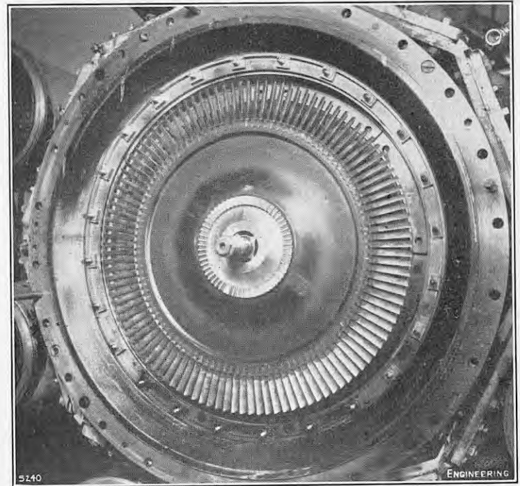
FIG. 7. SECOND-STAGE ROTOR OF COMPRESSOR TURBINE.
