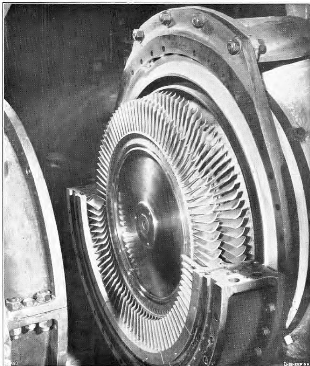
FIG. 8. POWER TURBINE; TOP-HALF STATOR CASING REMOVED.
