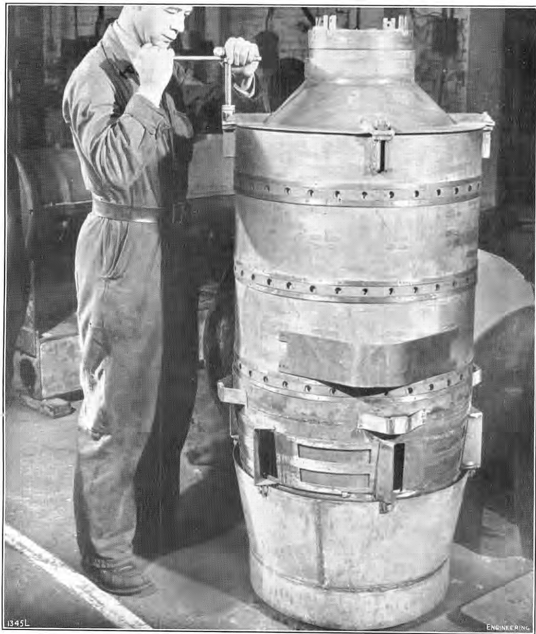
FIG. 5. INNER LINING OF LOUVRE-WALL COMBUSTION CHAMBER.
