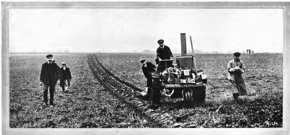
THE ROYAL AGRICULTURAL SOCIETY'S TRIAL OF AGRICULTURAL MOTORS AT MANOR FARM, BYGRAVE, BALDOCK, HERTS. —One of the competing machines—the Ivel—ploughing a 5-acre patch. This machine accomplished the work in 7½ hrs. and a similar one in 8 hrs.
