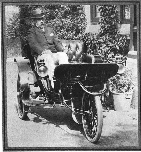
The three-wheeled 10 h.p. Duryea which took first prize in Class C in the Phoenix Park speed trials.
